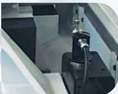
Tool measurement with table probing system (UCP 600)
