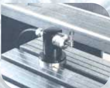
Tool measurement with table probing system (VCP 600, VCP 800)
