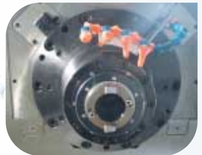
12,000 RPM spindle (ISO 40) with 4 adjustable coolant nozzles
