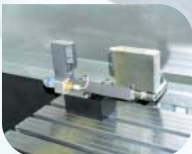
Tool measurement with laser control (VCP 600, VCP 800)
