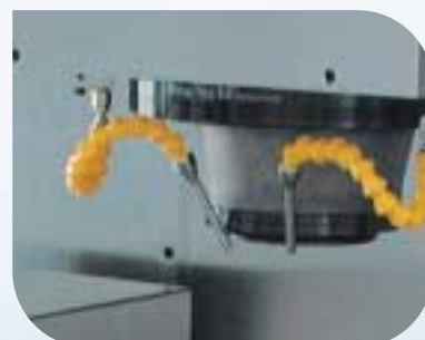
Minimum-quantity lubrication system (VCP 600, VCP 800, UCP 600)
