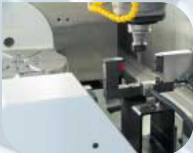
Tool measurement with laser control (UCP 600)
