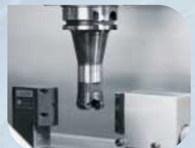
Monitoring accuracy: laser measurement can be installed.
